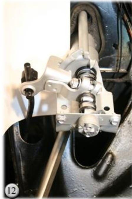
After bead-blasting the shifting mechanism and springs at the end of the column, it can be reassembled with a spring on each side of the shifter arm in the center. Notice the rod underneath the shifting mechanism is coming out at an angle. This is the steering shaft to the rack.
