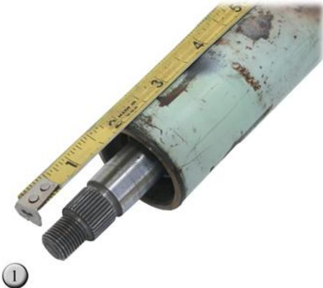
The first thing to do while the column is still in the car is to remove the steering wheel and measure from the top of the threads down to the top of the column tube. You should have 1 15/16-inches left for the steering wheel to go back in the correct position.
