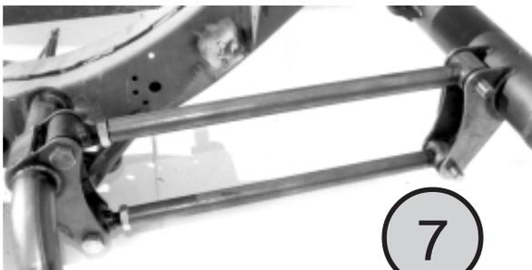
*Adjust each of the bars with 4 threads showing (#6) before assembly. When installing, the forward bolt heads face the inside while the rear bolt heads face outward.*
