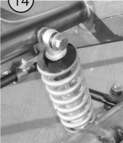
*The upper coilover shocks mount on the front of the rear tubular crossmember. They require a 5/8 - 18 x 2 1/4" bolt. The shock is sandwiched between two - 5/8 AN washers, with one star washer on the outside. Torque to 60 ft. lbs.*
