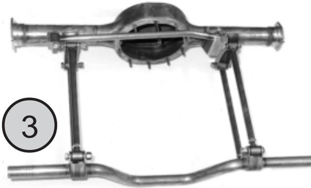
*All the brackets should be tacked onto the housing. Before you trim the forward 4-Link crossmember, install the 4-Links to the housing and front crossmember. Next, locate the rear axle centerline. Place the assembly under the chassis and center the housing on your centerline. Now you can measure and trim the forward 4-Link crossmember. Disassemble and tack the forward crossmember into position.*
